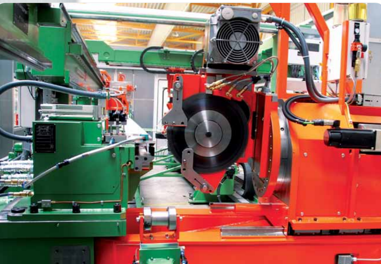
Double-angle saw with two swivel axes and a feed axis for HSS and hard metal blades
