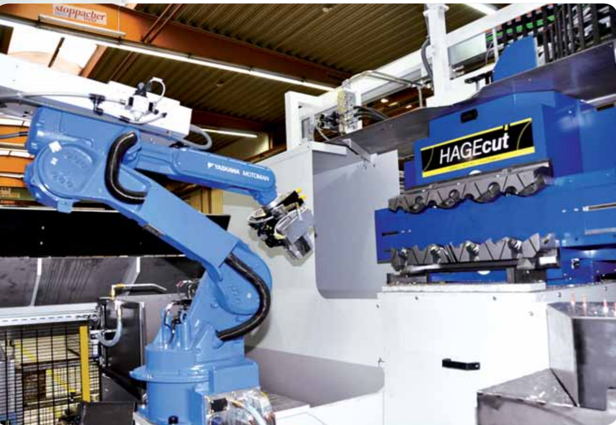
Robot loading and unloading workpieces. Clamp unit mounted on 180° swivel table.
