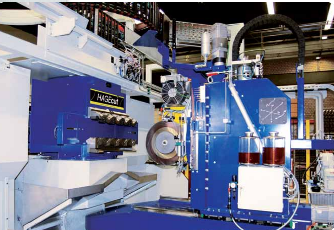
5-axis saw, NC-controlled, Double-angle saw with four positioning axes (two swivel axes (B, C) and two linear axes (X, Y), and a feed axis.
