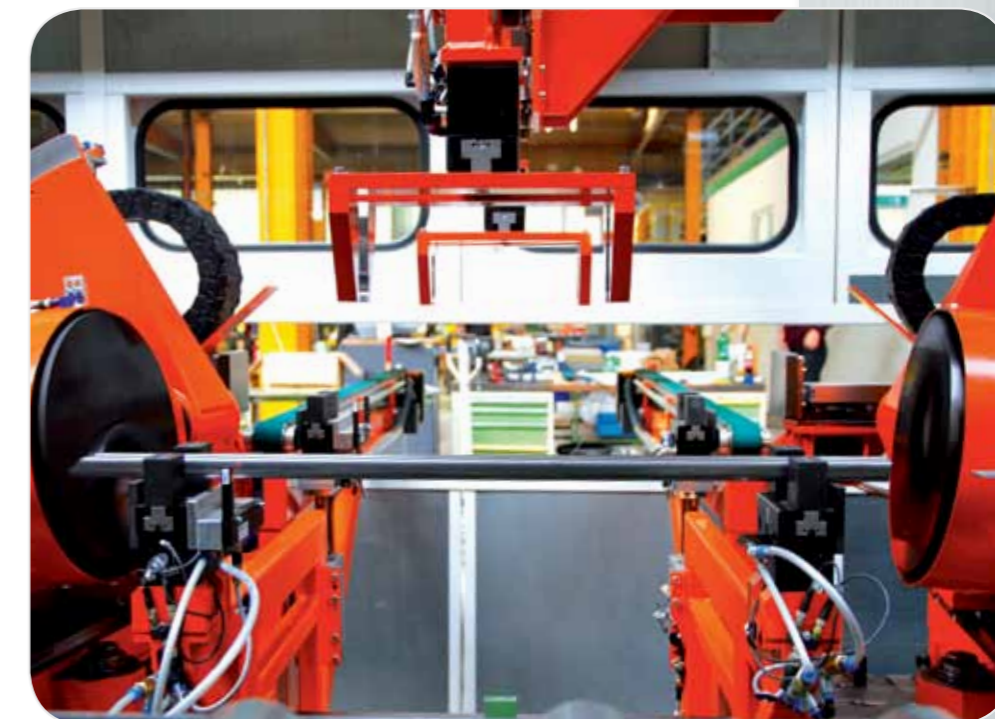
NC brushing and deburring station. The brush aggregates are automatically set to the appropriate cut angle and section length by two swivel axes and a linear axis.
