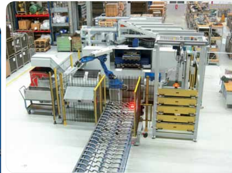
Loading belt: Manual adjustment to different workpiece dimensions
