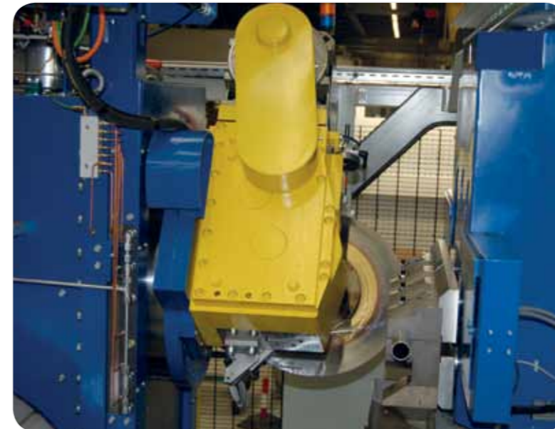
Excellent running properties thanks to an 11kW saw gear. Optimised durability by means of extremely small tooth-edge play on the drive (<4 angular minutes). Chiefly HSSE saw-blades used, but also HM saw-blades.
